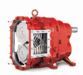
The combination of powerful shredding, easy-to-maintain design and long service life has made the XRipper XRS a reliable fixture in industry, production plants and sewage treatment plants. It reliably shreds entangled materials in sewage treatment plants: sanitary items, textiles and clothing in the wastewater of mixed sewers as well as bones, fruit, vegetables and food remnants in industrial and commercial applications.
