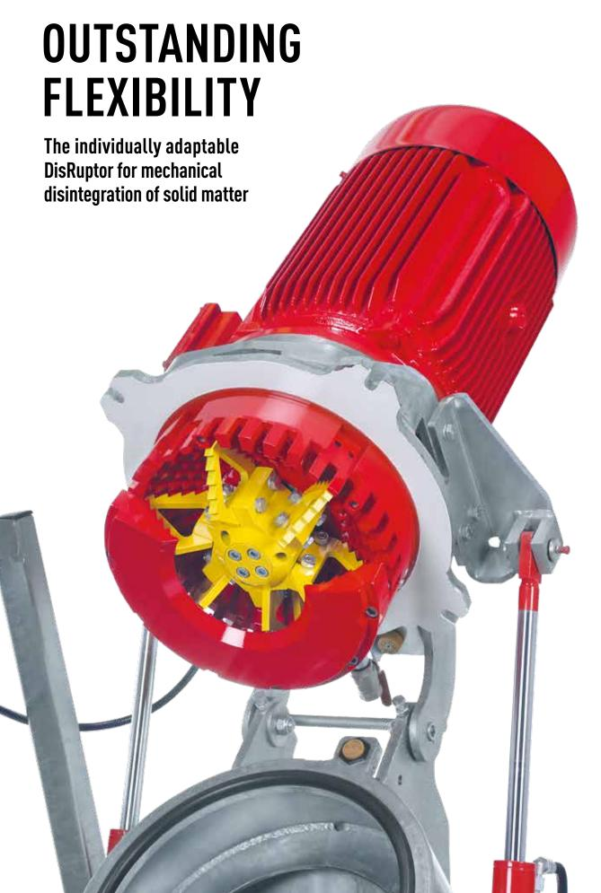
Optimal substrate disintegration is key for determining biogas yield. This is why Vogelsang also offers a mechanical alternative for disintegrating substrates: the flexibly designed DisRuptor. The reduction of the particle size and the simultaneous defibering increases the surface area of the solid matter used. This helps bacteria reach the nutrients better, accelerates conversion and increases the gas yield.
