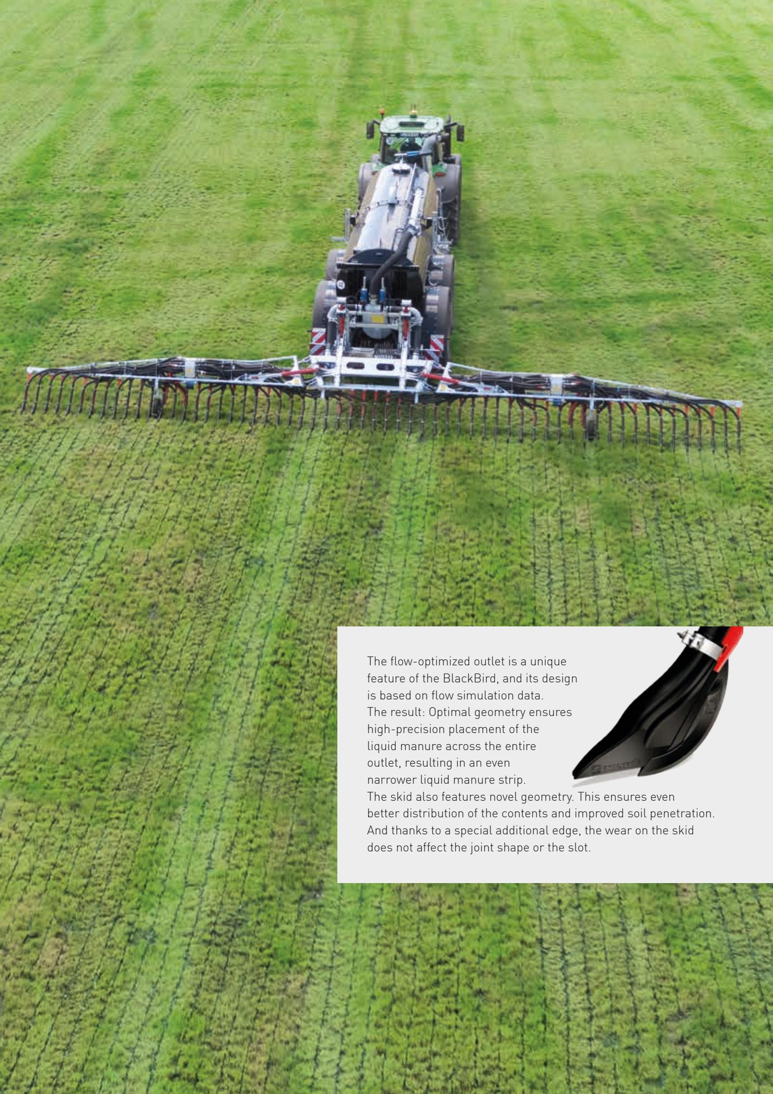
The flow-optimized outlet is a unique feature of the BlackBird, and its design is based on flow simulation data.
