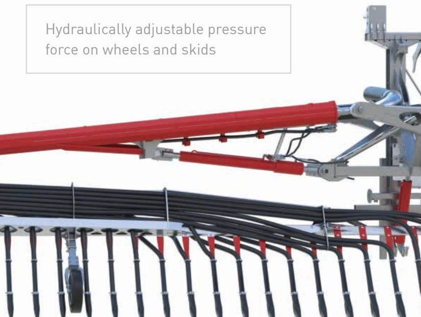
Flexible management of boom part width sections to implement different working widths with one linkage, without any overhang of the frame
