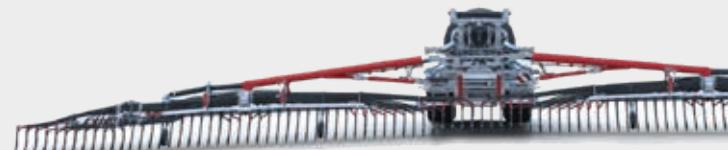
**Situation 2:** The tanker is located at the edge of a slope. The left side arm is positioned sloping down while the right side is in the horizontal position. The integrated height and pendulum compensation of the left cantilever compensates for the unevenness. All skids therefore follow the soil contour throughout.
