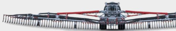
**Situation 1:** The tanker is located in a depression. The surface rises to the right and to the left. Thanks to its cantilever, the BlackBird can also adapt effortlessly here: each side arm compensates independently for the respective lateral height increase.
