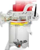
The medium flows steadily through the RotaCut macerator. Foreign matter (stones, metal parts, etc.) is separated out based on its size or weight and can be easily disposed of later via a cleaning port. All floating and suspended substances within the medium (fibers, hair, bones, wood, etc.) are transported to the cutting screen by the liquid flow and chopped by rotating, self-sharpening blades.
