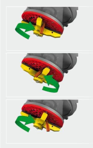
Thanks to the Auto-Reverse function, the system detects any blockage in the cutting head and reverses the rotational direction of the blade rotor. This process is repeated until the blocking matter is macerated.
