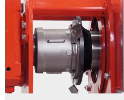
VarioAdjust hydraulic adjustment: The hydraulic pressure in the adjustment is adjusted by means of a hand pump, whereby the contact pressure adapts to the medium.
