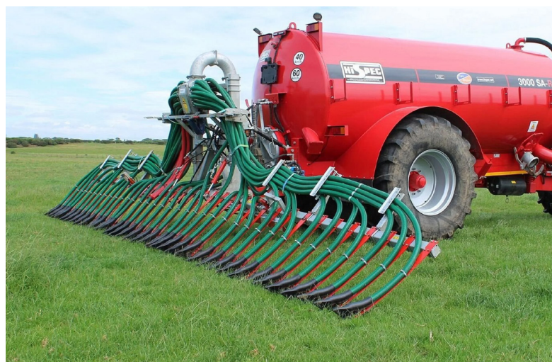
9 m UniSpread trailing shoe system
