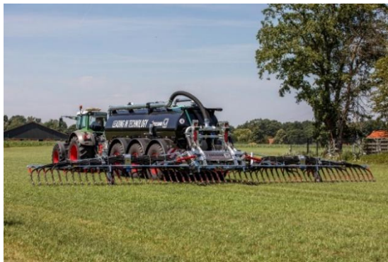
Image 7: The BlackBird Pro trailing shoe linkage, here in a working width of 15 meters.
