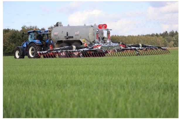
Image 6: The BlackBird Light is equipped with two ExaCut ECM distributors without air suction.
