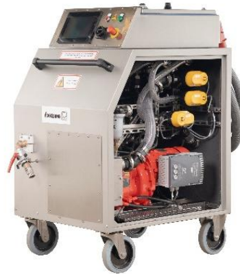
Image 4: The BioUnit MID is suitable for cleaning bioreactor toilets.
