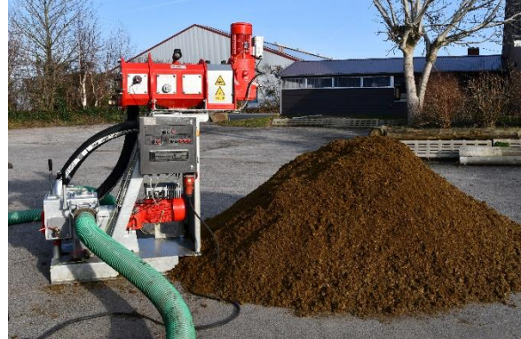
Image 4: The XSplite Compact separator reliably separates liquid manure into a solid phase and a liquid suspension.
