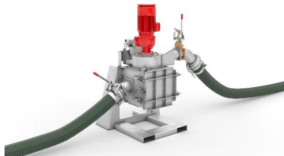
Image 2: The stand-alone RotaCut FillGuard is used for separating foreign matter before it reaches the slurry conveyor and, at the same time, shreds long-fibred feed and straw residues.
