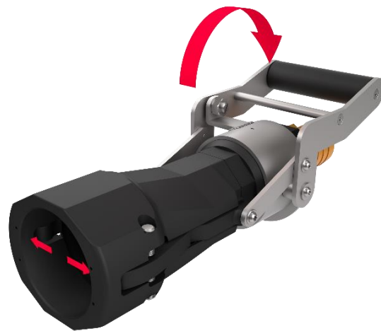
Image 2: When the lever is pulled back, the small locking elements detach from the connection piece on the tank and release the coupling.
