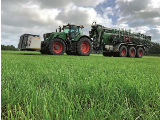
Image 3: SyreN is a closed system that stabilizes the liquid manure and reduces nitrogen losses. The added sulphuric acid is kept in a front tank and is fed into the liquid manure stream in a mixing chamber upstream of the spreading linkage.
