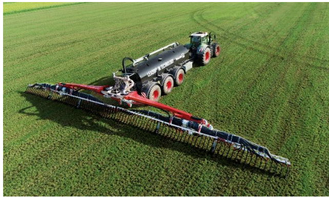
Image 2: With a working width of 24 meters, the BlackBird trailing shoe system places the liquid manure precisely at the plant.
