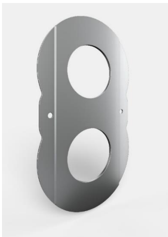
Image 5: Pump technology: The modified wear plate keeps fibrous matter away from the seal. This serves to extend the service life of the seal up to four times.
