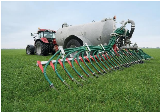
Image 1: The UniSpread has a compact design and can be combined with various liquid manure outlets (here: trailing shoe).
