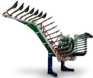
**Image 3:** UniSpread in the folding process: the universal linkage is now available in a working width of 10.5 meters.
