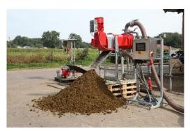
**Image 2:** The new XSplit press screw separator achieves dry matter content of up to 40 percent.
