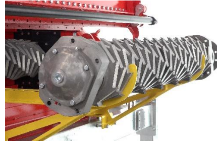
Image 2: A removed ripper on the assembly aid.
