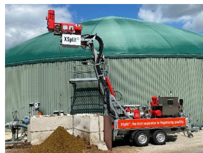
Image 4: XSplit press screw separator: innovative separation as a system solution (shown) or individual component.
