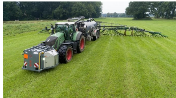
Fig. 4: Liquid manure acidification in field distribution with SyreN (here in combination with the SwingMax dribble bar linkage system).
