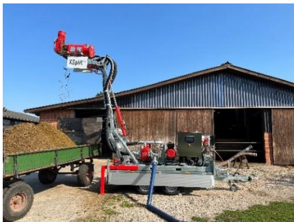
Fig. 3: XSplitt press screw separator as a system solution with pump and control technology.
