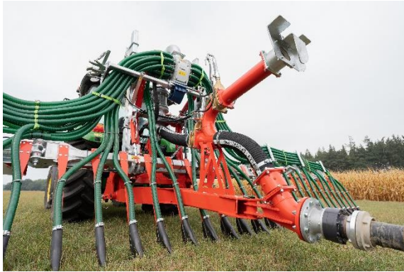
Fig. 1: The UniSpread universal linkage (here with trailing shoe technology) as a hose version with liquid manure supply hose, patented swivel spout including swivel joint and mounted distributor head.
