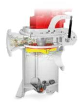
The medium flows steadily through the RotaCut macerator. Foreign matter (stones, metal parts, etc.) is separated out based on its size or weight and can be easily disposed of later via a cleaning port. All floating and suspended substances within the medium (fibers, hair, bones, wood, etc.) are transported to the cutting screen by the liquid flow and chopped by rotating, self-sharpening blades.
