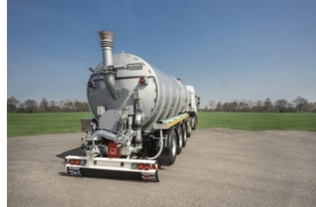
Image 4: In action: aluminum pump on tank trailer for liquid manure transport.
