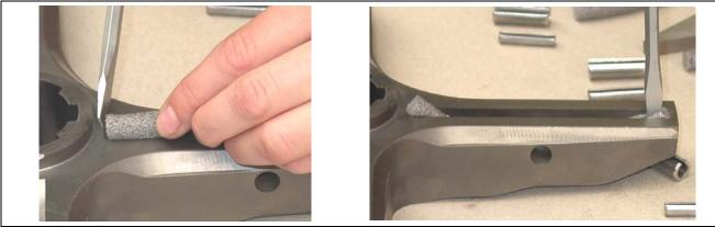
Fig. 11: Preparing the blade rotor for installation of the blades
