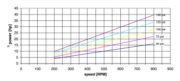
Values based upon water 70°F <sup>1)</sup> required driving power at the pump shaft
