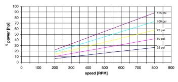
Values based upon water 70°F 1) required driving power at the pump shaft
