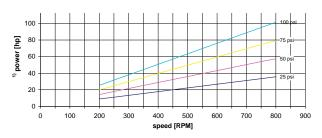
Values based upon water 70°F  $^{1)}$  required driving power at the pump shaft
