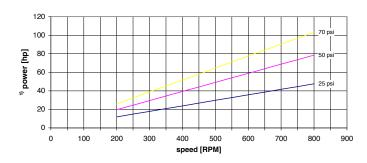
Values based upon water 70°F 1) required driving power at the pump shaft
