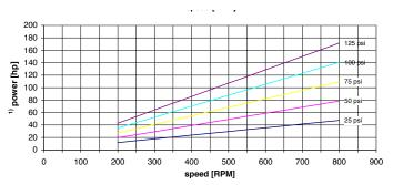
Values based upon water 70°F <sup>1)</sup> required driving power at the pump shaft
