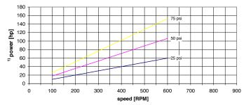
Values based upon water 70°F <sup>1)</sup> required driving power at the pump shaft
