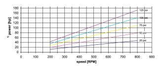
Values based upon water 70°F <sup>1)</sup> required driving power at the pump shaft
