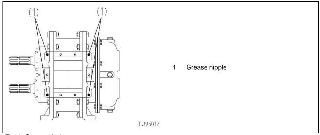
Fig. 8: Grease nipple
