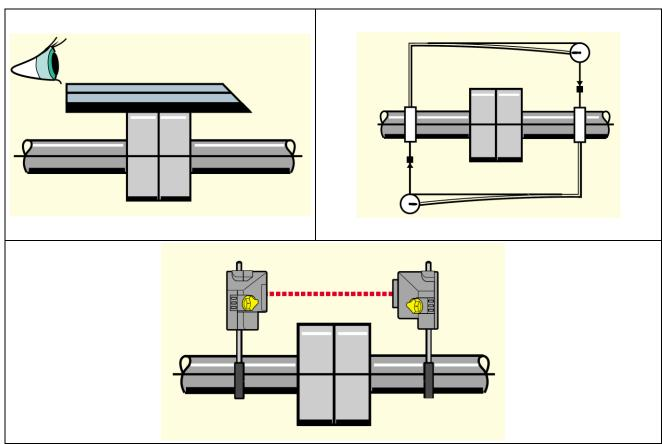
Fig. 2: Alignment methods
