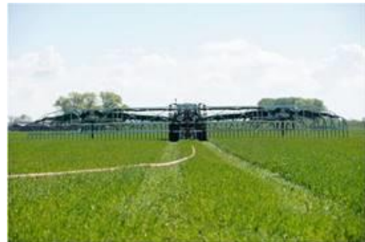
Image 2: The integrated pendulum compensation allows the user to optimally align the slurry distribution to the existing ground contour.
