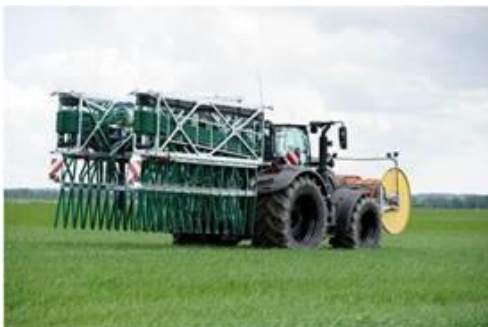
Image 3: With a compact transport width of 2.55 meters, driving on roads remains uncomplicated.
