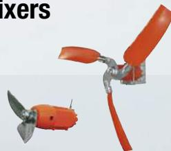
Submersible mixers are used in digesters to mix and homogenise the substrate, thus increasing the output of the plant and prevent solids settling down which in the long run might reduce the efficiency of the plant, for instance by clogging its pipes.
