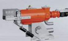
Separators are used to separate the solid fraction from the liquid in the anaerobic fermentation process. The liquid fraction can be used as a fertiliser and for irrigation. The solid fraction may be used as an amender, as cattle beds, etc.. Use of separators is also recommended as a pre-treatment in nitrogen-reducing plants.
